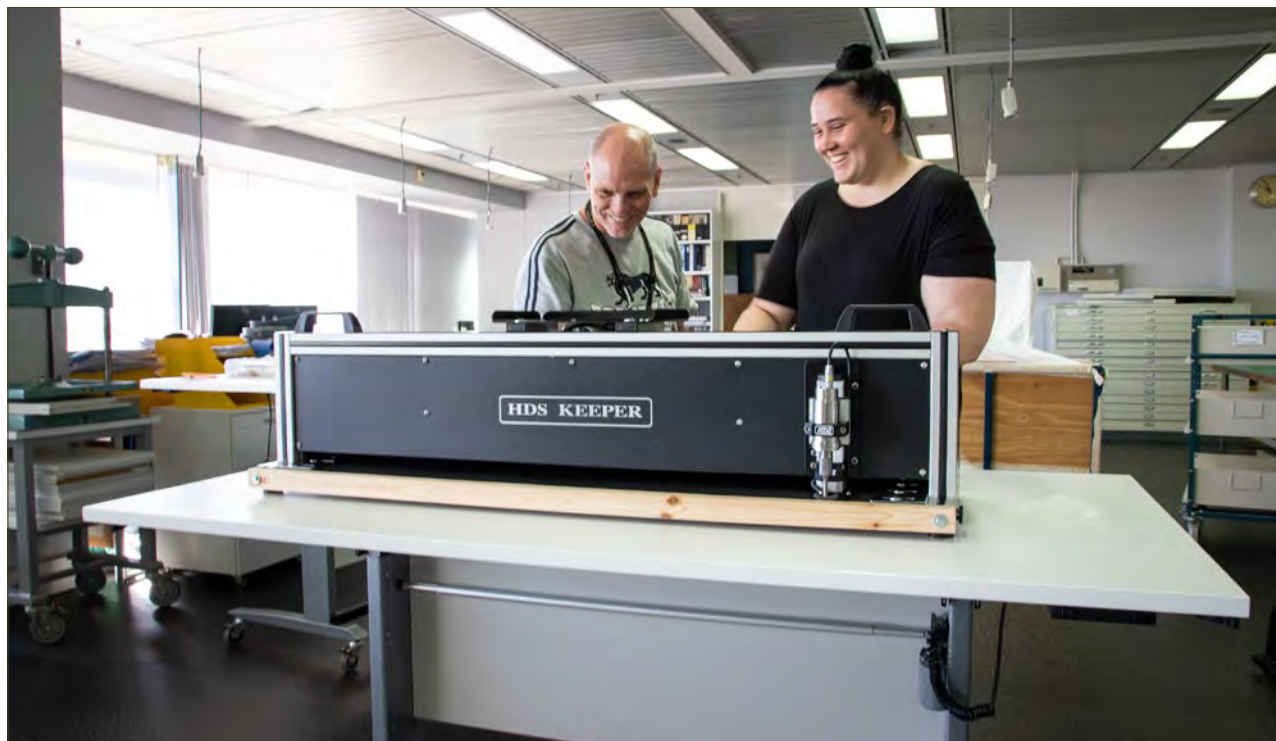
State Library staff unbox a new ultrasonic welder in the State Library Conservation Laboratory, May 2018. An ultrasonic welder is used to create custom housing for fragile collection items
